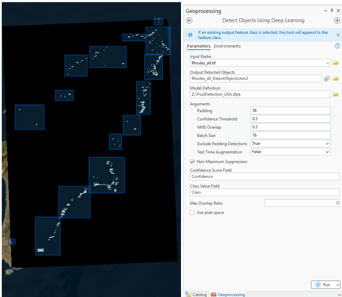
Figure 2: Sub-divided areas for Object detection (left) and Object detection settings (right) used
